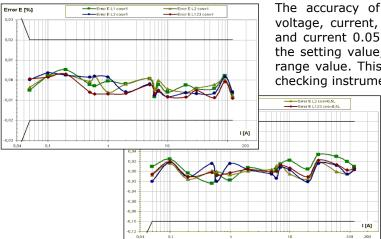
The accuracy of the basic parameters of the Calmet TB30 voltage, current, power and energy in a wide voltage 21...560V and current 0.05...120A ranges, is expressed as a percentage of the setting value, without the component as a percentage of the range value. This form of errors specification is very useful when checking instruments, such as electricity meters.
