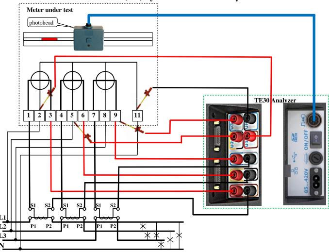
CAUTION! During making brake on secondary side of CT to connect TE30 directly, shunt the S1 and S2 terminals <u>BEFORE BREAK</u> and after connection to the TE30, remove shunt.
