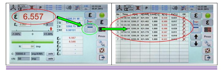
Testing the error of 3-Phase 4-Wire Energy Meter, connected by Current Transformer (CT) by means of TE30 Analyzer.
