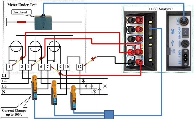
After Clamps, Measurement and Power supply cables connection TE30 analyzer is READY to work. **REMARK! The best measurements results are at the Power network Load > 500W.**
