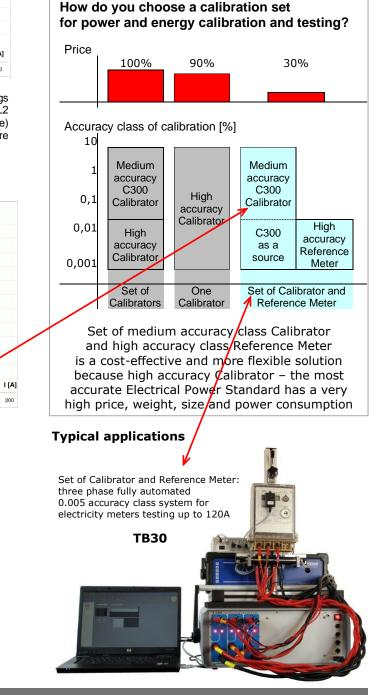
The most reasonable solutions for a 0.02 and 0.005 accuracy class in power and energy calibration
