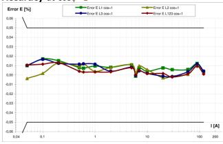
Energy error diagrams of the C300 as a function of current settings in 0.05...120A range for balanced L123 and unbalanced L1, L2 and L3 loads at 230V/50Hz and power factor  $\cos\varphi$ =1 (top figure) and 0.5L (bottom figure), achieved in automatic test procedure using Calpro300TS software and reference meter Radian RD31
