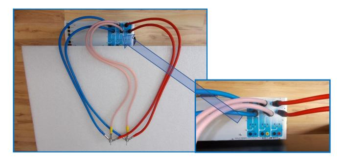
The sequence of assembly: screw, washer, terminal, terminal, terminal (ring), washer, nut.
