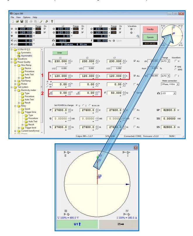
After performing the above mentioned steps, the parallel connection of C300B current outputs will be achieved and an output current of up to 360A will be generated.
