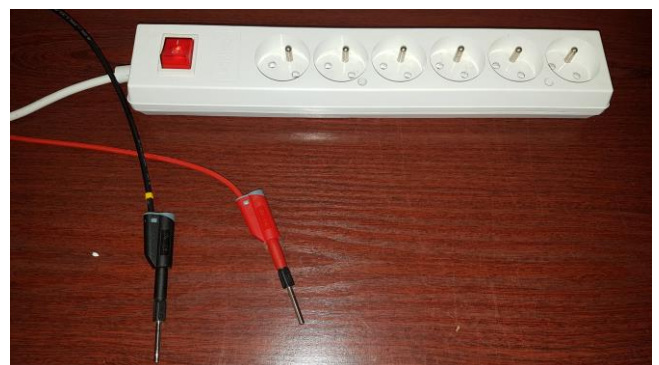
Prepare the other side of TE30 Lite connection cables for connection to the measured circuit
