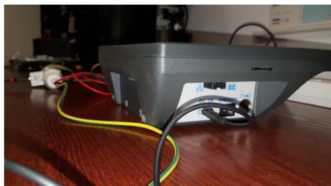
Connect power supply plug to DC IN of TE30Lite
