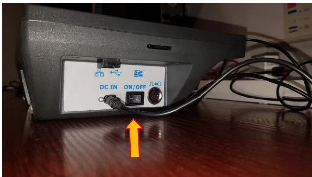
Connect supply to TE30Lite and switch it ON
