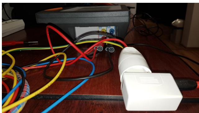
Insert the TE30Lite power supply to the AD100EXT socket
