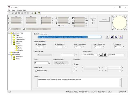
2. The Procedure function allows the user to prepare a set of load points acc. to requirements of standard (in this case acc. to EN 50470-3) or acc. to the individual requirements of the user.
