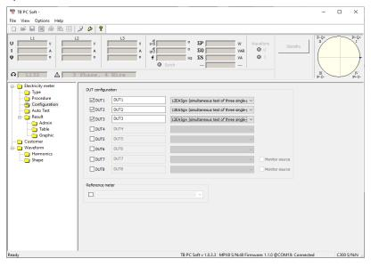
4. The AutoTest function takes the load points acc. to the procedure are generates them automatically. For each load point, the accuracy of the energy meter under test is calculated.
