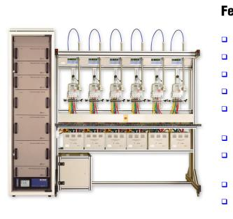
The ASTeL 2 meter testing system is a fully automatic system enabling simultaneous, multiposition calibration and legalization of single-phase and three-phase electric energy meters. The automatics include power sources, reference standards, stand controllers, photoelectric scanning heads, separating transformers and other elements of the system. All these elements are controlled through a Windows<sup>®</sup> based executive program.
