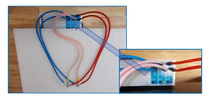
Details of connection. The sequence of assembly: screw, washer, terminal, terminal, terminal (ring tipes), washer, nut.
