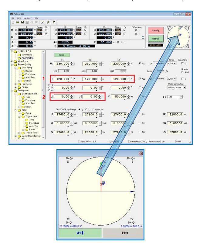
After performing the above mentioned steps the parallel connection of C300B current outputs will be achieved and output current up to 360A will be generated.
