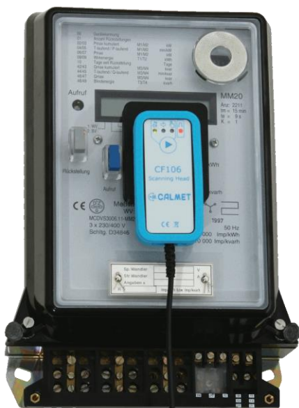
Test of electricity meter with LED (scanning head mounted using EH01 Handle by self adhesive Velcro – CF106V )
