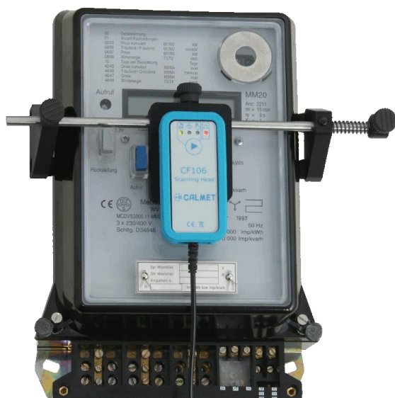
Test of electricity meter with LED (scanning head mounted using UCF106 Holder – CF106H option )
