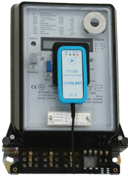
Test of electricity meter with LED (scanning head mounted using EH01 Handle by self adhesive Velcro)
