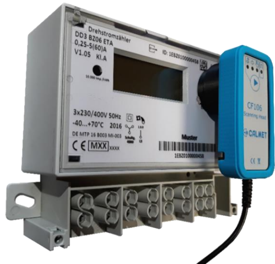
Test of electricity meter with LED (scanning head mounted using EH02 Magnetic handle – CF106M option )
