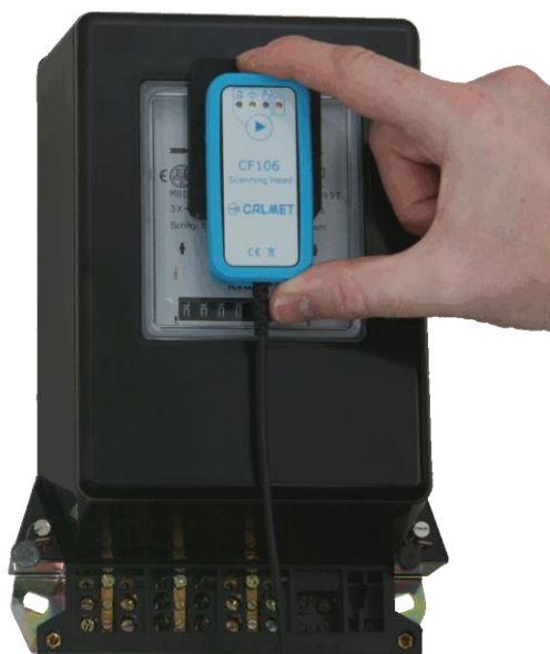
Quick test of electricity meter with rotor (work „by hand” without mounting to meter)
