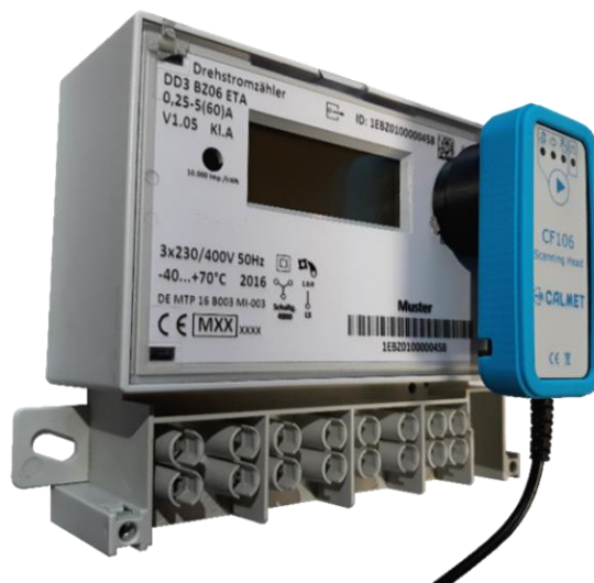
Test of electricity meter with LED (scanning head mounted using EH02 Magnetic handle – CF106M option )
