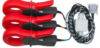
Current clamps CT1000AC allow for easy current measurement on cables and bars in electric installation. Due to narrow jaws and large hole diameter, it is easy to assembly them in hard access places. Maximum diameter of cable, on which we can close the sensor is about 52mm.
