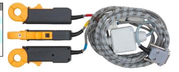
Current clamps CT100AC allow for easy current measurement on cables and bars in electric installation. Due to narrow jaws and large hole diameter, it is easy to assembly them in hard access places. Maximum diameter of cable, on which we can close the sensor is about 15mm.
