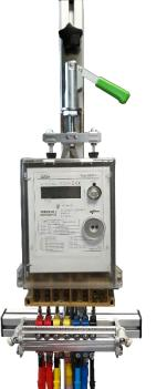
Spring contact pins of the EH10.3 are used to make connection to the meter and may be easy moved sideways and fixed in any desired position with distance between two adjacent contact pins from 14mm. It is also easy to remove and switch the pin positions for preparing the contact pin configuration to many different meter connection schemes including single and three phase meters.
