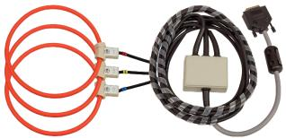
Flexible current clamps (Rogowski coils) FCT3000AC.B allow for easy current measurement on cables and bars in electric installation. Due flexibility and small sensor diameter it is easy to assembly them in hard access places. Maximum diameter of cable, on which we can close the sensor is about 150mm.
