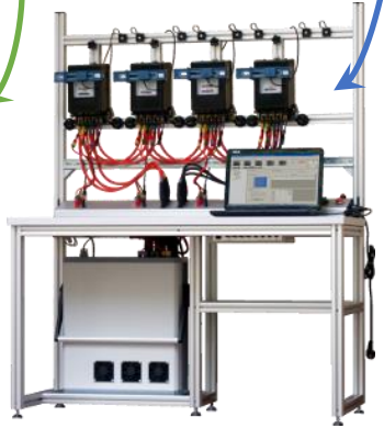
TB40 560V 120A up to 4 positions class 0.02&0.05
