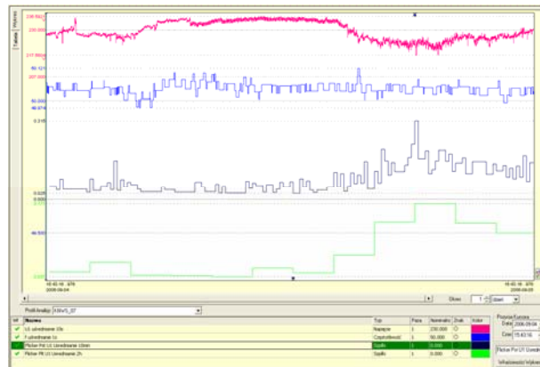
Rys.9. Okno programu na komputer do analizy zmian flikera. Fig. 9. PC computer screenshot with analysis change of flicker.
