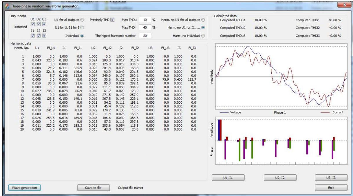
Fig. 4 The screenshot of the front panel of the realized virtual random wave generator.
