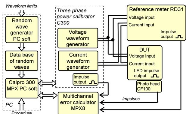
Fig. 2. Block diagram of the realized multi position fully automatic test system for simultaneous testing of several energy meters with reference to the power calibrator or the reference meter.
