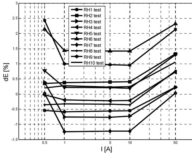
Fig. 13. The characteristics of the EEM additional error for ten standard signals (PF=1∩bal.).
